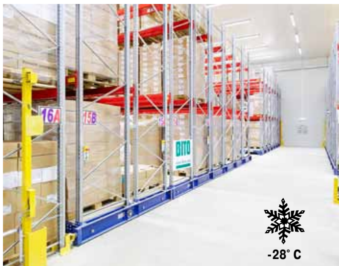
Mobile pallet racking operated in a deep-freeze environment
