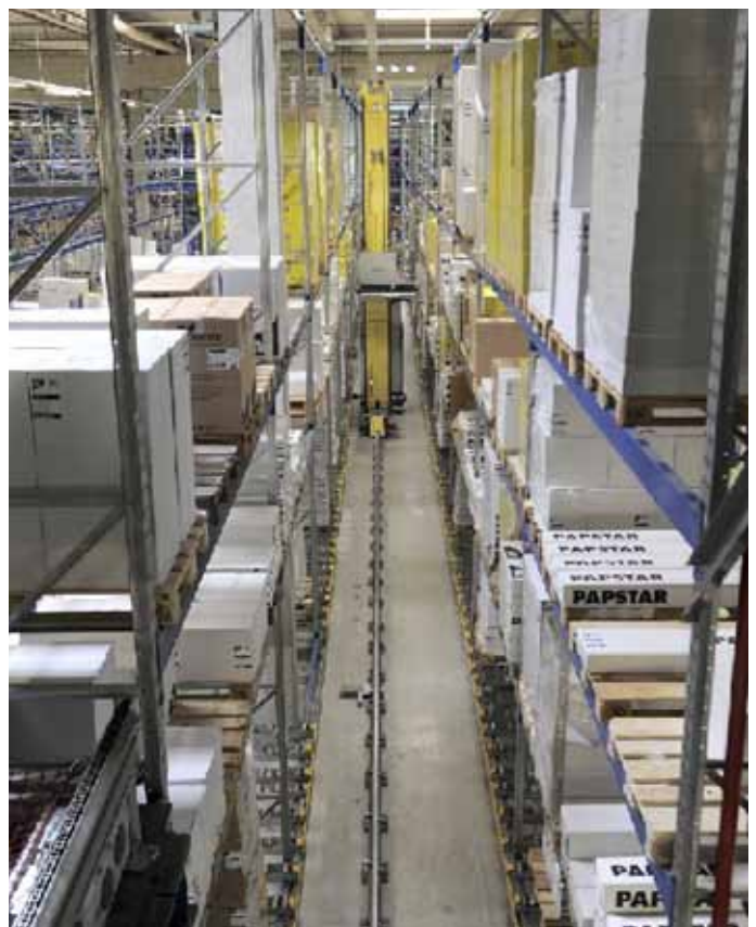
Pallet racking being loaded at Papstar. At floor level height, pallets are loaded into live storage lanes to supply the order picking area.
