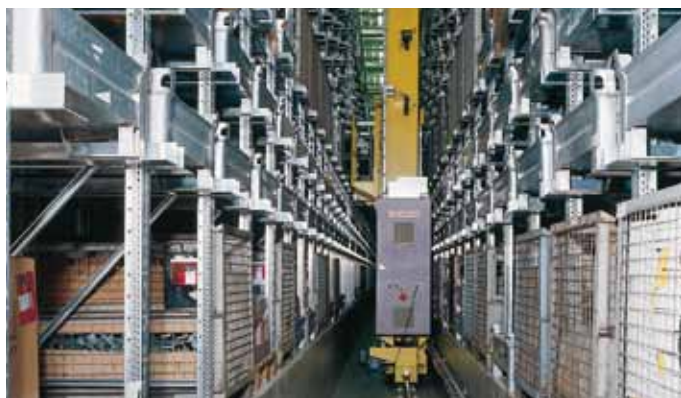
Automated pallet racking with single position storage
