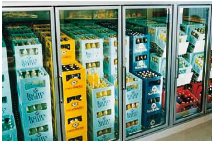
Lanes with inclined picking tray facilitate picking of individual bottles, straight lanes are suited for picking complete cases.
